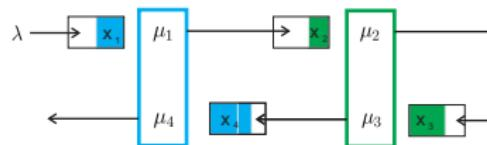
$$\dot{x}(t) = V_{q(t)}, \quad \text{например} \quad V_{(1,3)} = \begin{pmatrix} \lambda - \mu_1 \\ \mu_1 \\ -\mu_3 \\ \mu_3 \end{pmatrix}$$
